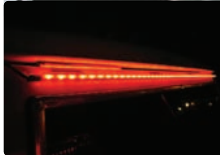
The LED light bar fits a Bronco hardtop like a factory option. At night, it shows the width of Bronco, and if you are stopping or turning.
