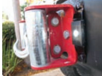
Sealed LED running lights or area illumination lights shown on and off
