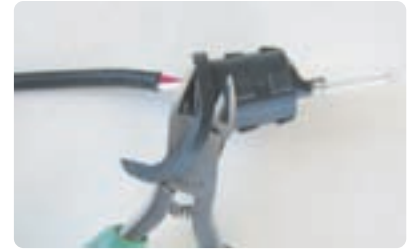
Trim the rubber flange off the strobe base
