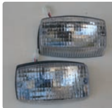
The clear plastic utility lights hold the front strobes. Look for the model without a switch and with a reflector.
