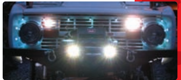
This shows the front strobe lights, the LED running lights, and some bottom illumination from the LED strobes. (There are also LEDs all around the perimeter of the grill, but that is a story for another time.)
