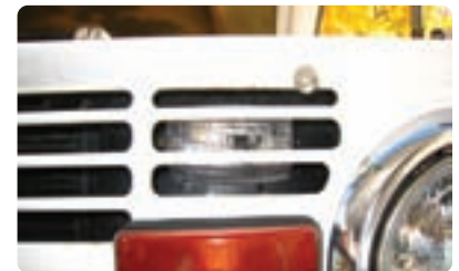
The modified utility strobe lights mounts handily behind the grill, just above the turn signals. Of course, you can put them most anywhere you want.
