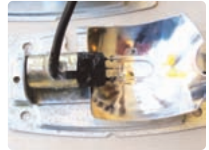
Silicon the strobe into the socket so it is off-road proof
