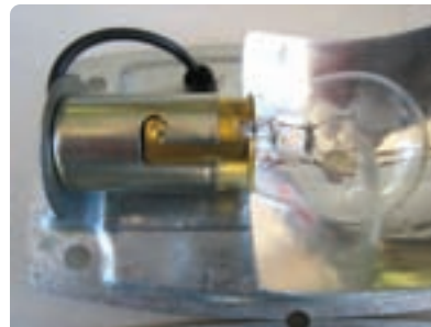
The clear plastic utility lights hold the front strobes. Look for the model without a switch and with a reflector.
