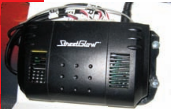
The StreetGlow controller module lets you pick any of a dozen or so different patterns.
