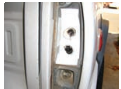
The rear strobes fit well in the tail light housing. You need a 5/8" hole. Mount the strobe low enough to clear the 1157 bulb or the Dakota Digital LED replacement. Wire everything up to the controller and blind - I mean Bling - your friends.
