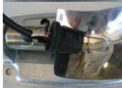
Remove the light bulb and file or Dremel the socket out to provide an exit opening for the strobe wires.
