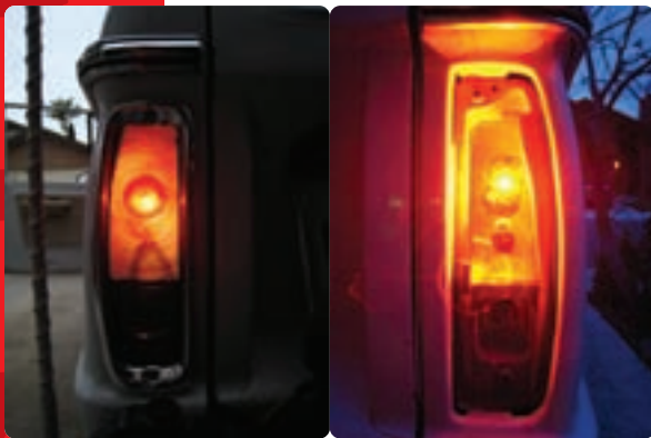
The LED in the bright mode (brake or turn signal), with and without the lens cover
